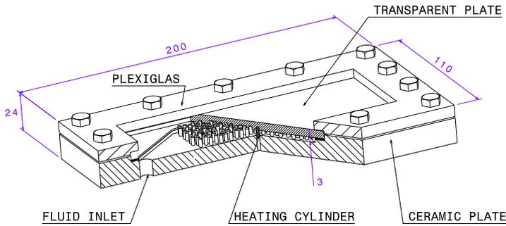
**FIGURE 3.** EXPERIMENTAL SETUP: TEST SECTION (DIMENSIONS IN mm).
