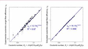
A dimensionless coulomb number,  $K_{\rm C}$  which is the ratio of the drift velocity due to coulomb attraction to the airflow velocity is proposed The Cunningham slip correction factor, C is included to account for molecular slip.
