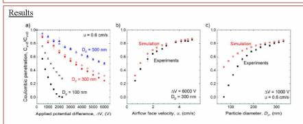
$P_{coul}$  decreases as the applied potential difference increases. This effect occurs because the attractive forces between the particles and fibers increase with greater applied potential differences.
