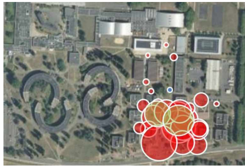
Figure 1. Helium measurements on 11 September 2020 between 5:35 and 06:05 UTC at Sirta. Emission point in blue, ATC at sampling in red point, and ATC at real time spectrometer in green point. The bubbles size is proportional to the ATC.
