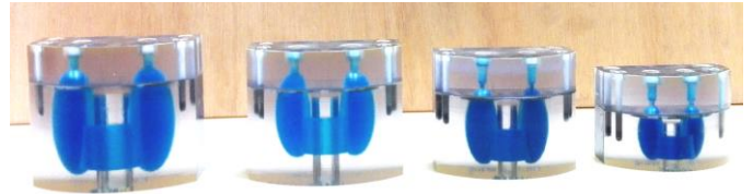
Figure 1. Age-specific thyroid phantoms corresponding to (left to right) an adult, 15 years-old teenager and 10 and 5 years-old children.
