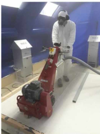
Fig. 7. Experiment of scarifying operations of a concrete slab using a manually propelled industrial milling machine [15]
