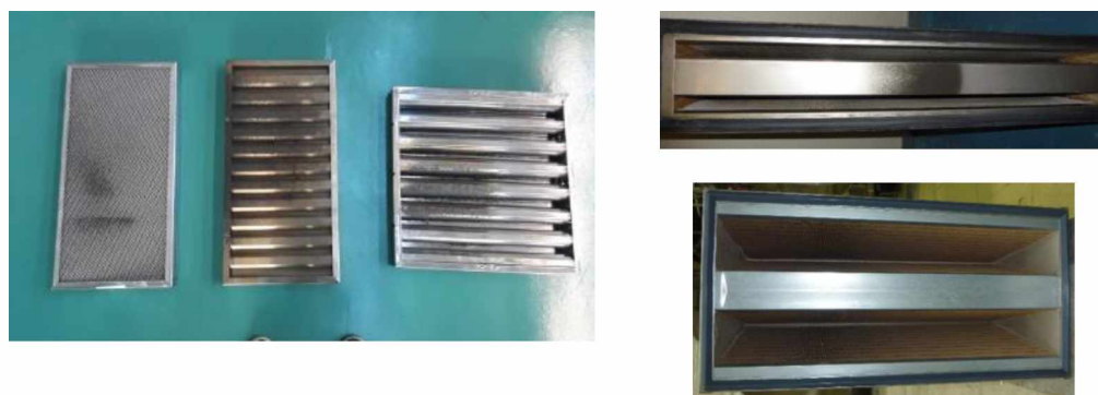
Fig. 14. (left) Three models of spark arrestors tested; (right) Two models of filters tested [22]
