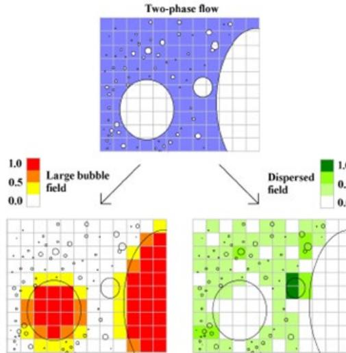
**Figure 2** Illustration of the multifield approach used to simulate a two-phase flow
