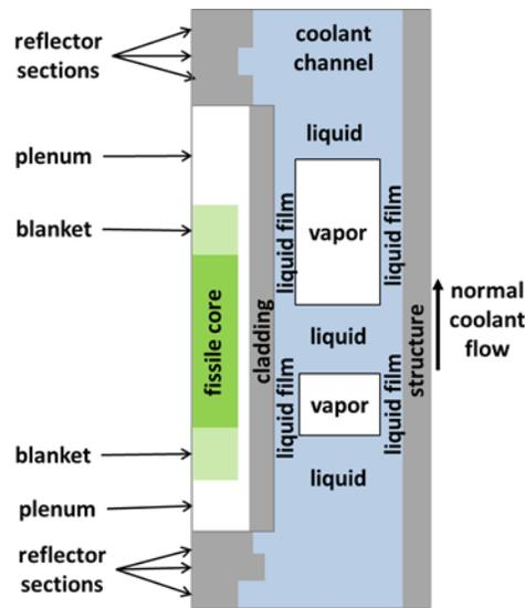
**Figure 1** Representation of the multiple-bubble boiling model
