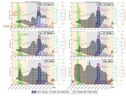
At this station, cloud thickness is very sensitive to the cloud diagnosis, contrary to the cloud presence. Relative humidity at 80% and LWC at 10<sup>-4</sup> Kg.m<sup>-3</sup> give poor performances.
